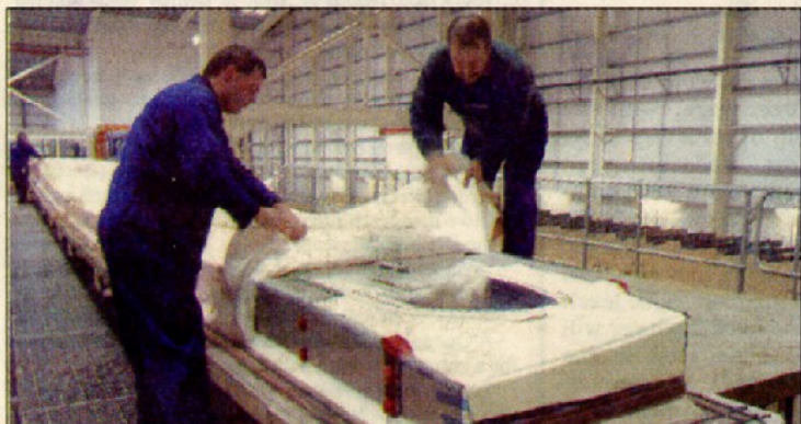
Removing protective material from a completed A380 wing skin section after forming on the new production system designed by Bennett Associates
