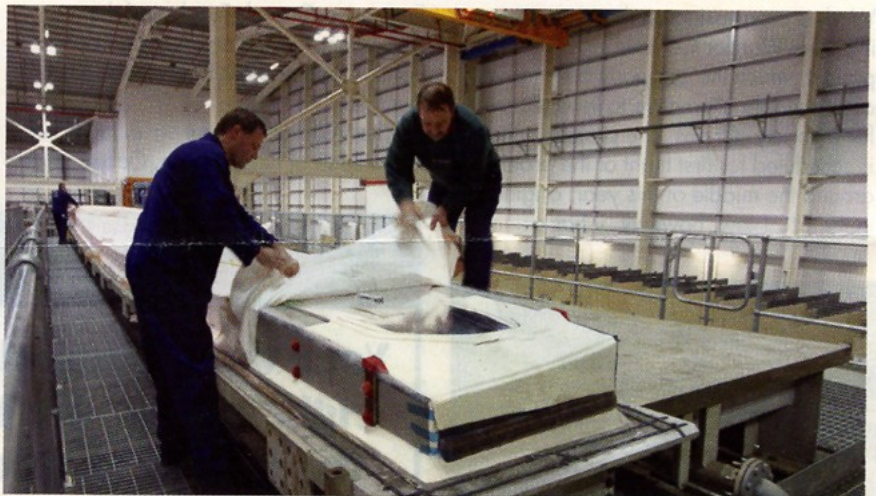
Airbus wing skin wrapping: the A380's upper wing skins are believed to be the largest components ever produced by the creep-forming process.
