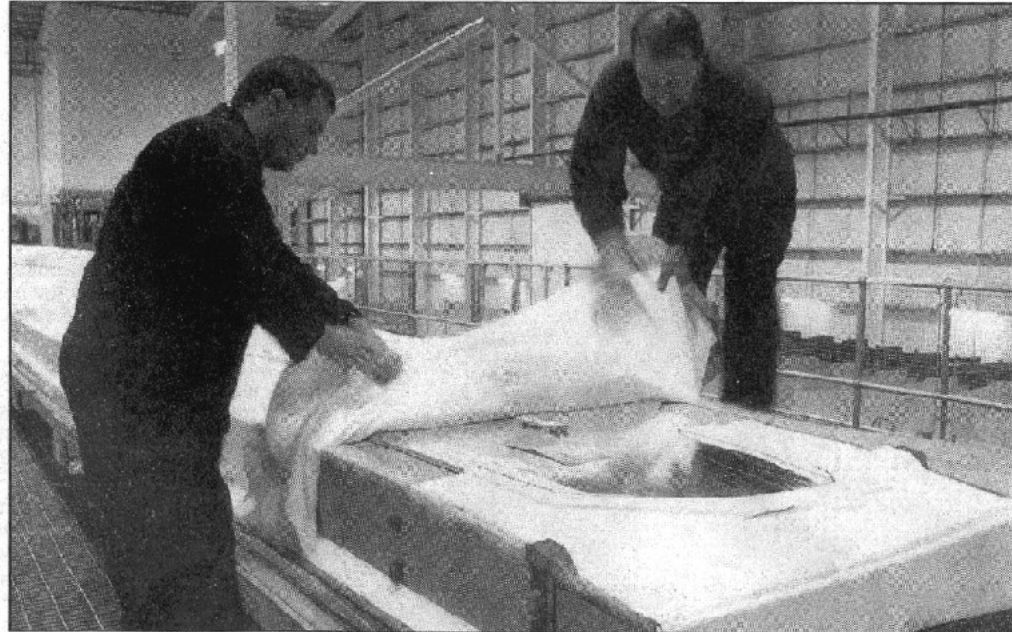
▲ Ready to fly: Removing protective material from a completed A380 wing skin
